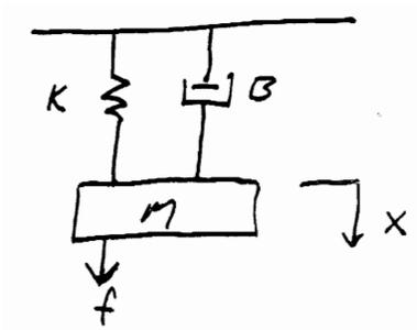
Suppose  $M, K$  are given. How should you choose  $B$  (shock absorber) so that the P.O. to a unit step is less than  $\sim 4\%$ .
