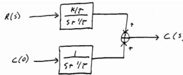
By superposition the response of the system is the sum of the response due to the initial condition alone (the *free response*) and the response due to the input  $R(s)$  (the *forced response*).
