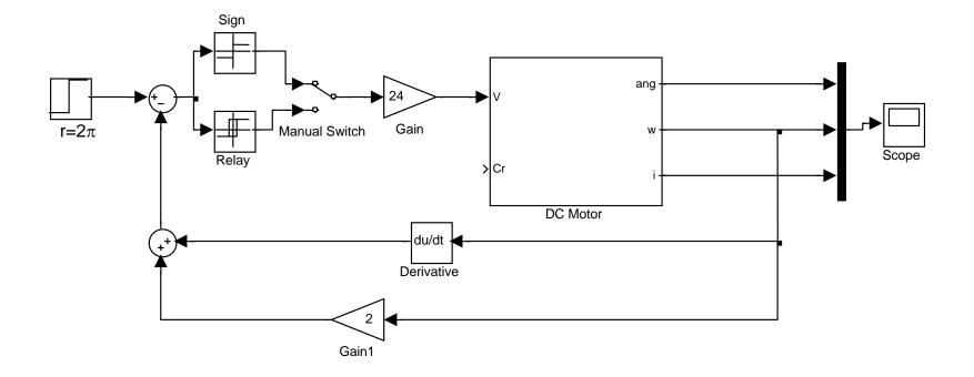
Take care that because of the feedback, the new closed loop gain (assuming the rotor velocity as the output) will be 1/2
