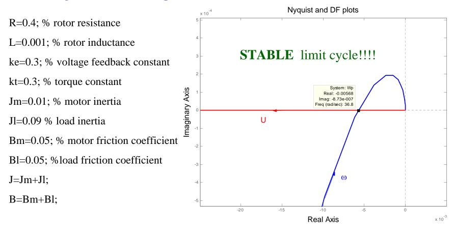
$$\omega|_{\mathfrak{I}(W_p(j\omega))=0} = \omega_{cr} = \sqrt{\frac{R_a B + k_t k_e}{L_a J}} = 36.056 \text{ rad/s} \qquad \overline{\mathbf{U}} = -\frac{4\mathbf{M}}{\pi} \cdot \mathfrak{R}(W_p(j\omega_{cr})) = 0.1759 \text{ rad}$$
