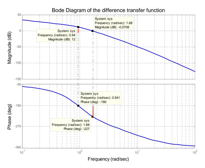
The NOT saturated system is not stable since its stability margin are negatives
