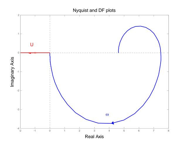
The Nyquist plot of the linear system **cross** the negative reciprocal of the DF at the origin, i.e., U=0 and  $\omega = +\infty$
