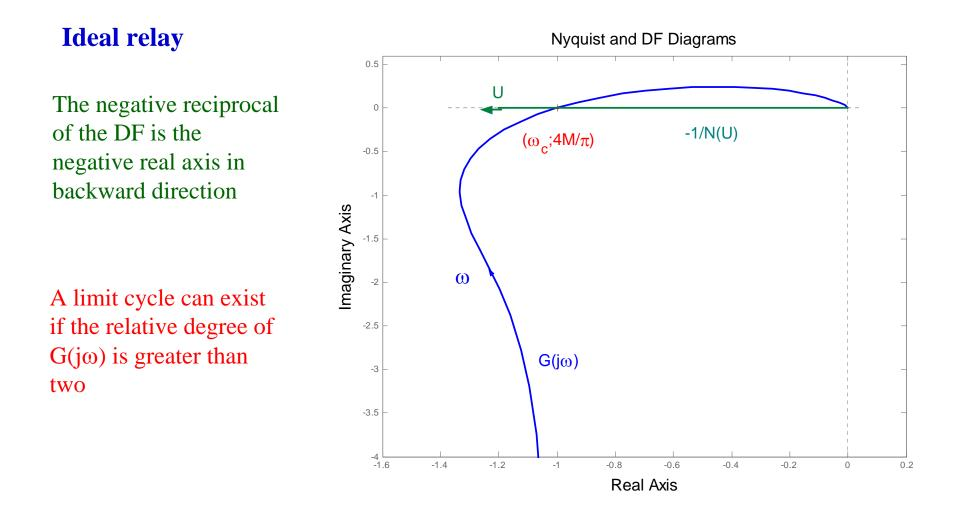
The oscillation frequency is the critical frequency  $\omega_c$  of the linear system and the oscillation magnitude is proportional to the relay gain M
