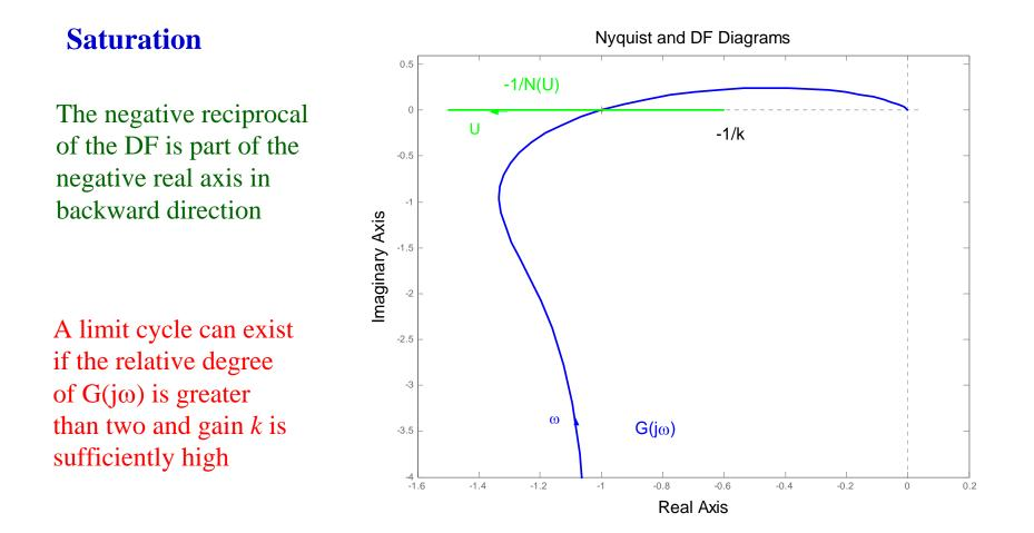
The oscillation frequency is the critical frequency  $\omega_c$  of the linear system and the oscillation's magnitude depends on the saturation parameters M and k
