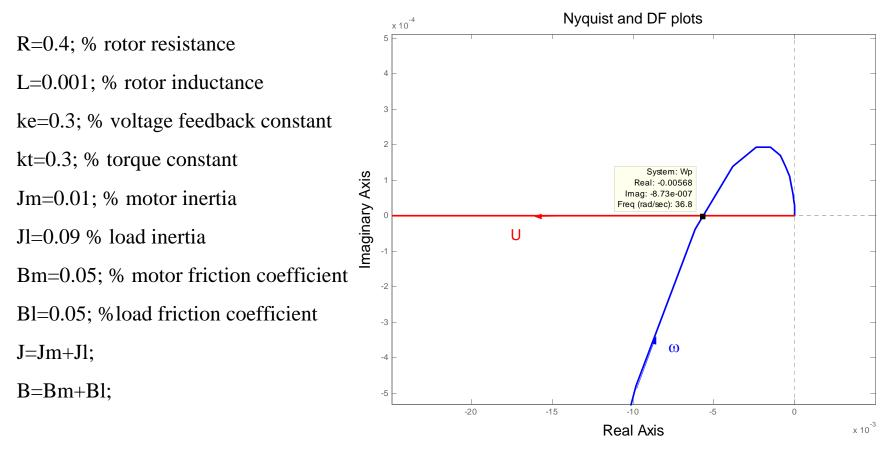
$$\omega|_{\Im(W_p(j\omega))=0} = \omega_{cr} = \sqrt{\frac{R_a B + k_t k_e}{L_a J}} = 36.056 \text{ rad/s} \qquad \overline{\mathbf{U}} = -\frac{4\mathbf{M}}{\pi} \cdot \Re(W_p(j\omega_{cr})) = 0.1759 \text{ rad}$$
