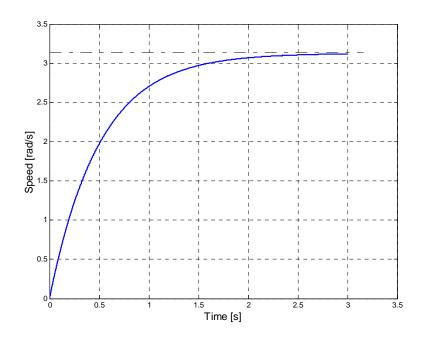
Apart from a very short transient, the state trajectory tends to the steady-state values sliding on a linear manifold of the state space It is apparent that the shaft speed tends to the steady state value  $\pi$  as a first order system with  $\tau = 0.5$  s
