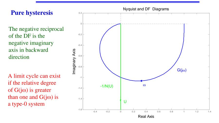
The oscillation frequency is lower than the critical frequency  $\omega_c$  of the linear system and the oscillation's magnitude is proportional to the relay gain M and to the modulus of the transfer function at phase  $-\pi/4$
