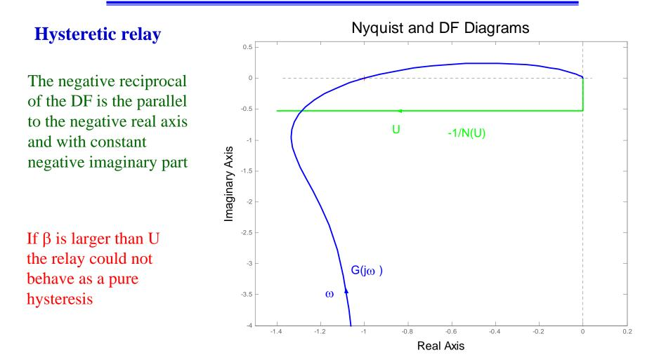
The oscillation frequency is lower than the critical frequency  $\omega_c$  of the linear system and the oscillation's magnitude is proportional to the relay gain M
