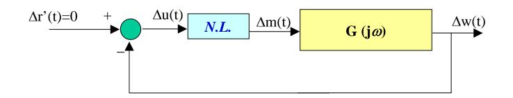
A permanent oscillation in the loop appears if  $\Delta u(t) = -\Delta w(t)$
