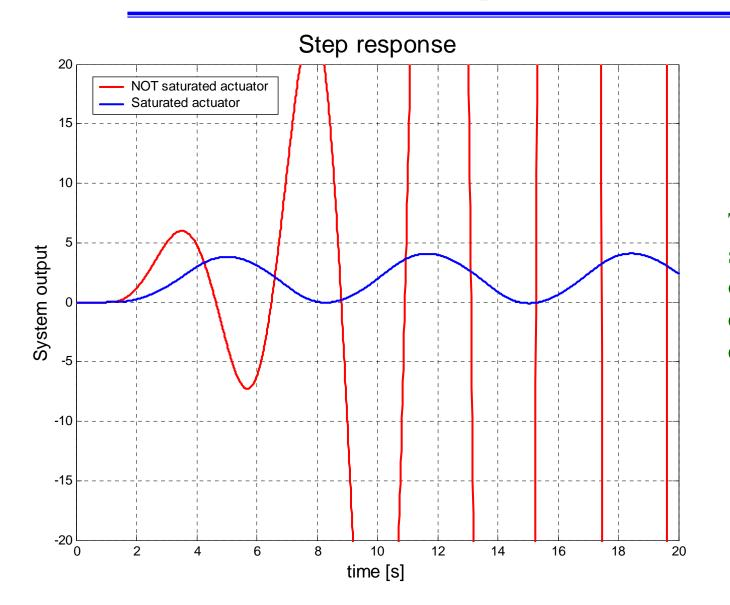
The saturated system oscillates but does not diverge
