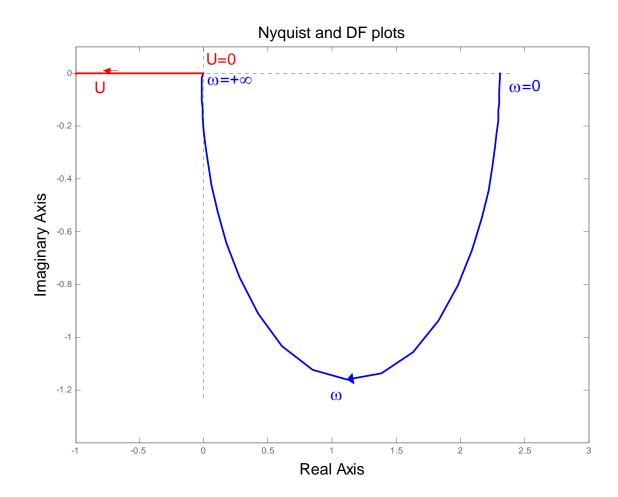
The Nyquist plot of the linear system is **tangent** to the negative reciprocal of the DF at the origin, i.e., U=0 and  $\omega = +\infty$
