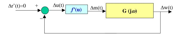
If f'(u) is a passive sector function **absolute stability** tools allow for **sufficient conditions** for global asymptotic stability of the variation system, i.e, the steady state is characterised by constant values of the system variables
