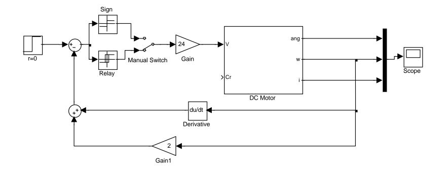
It is apparent that an ideal sliding mode cannot appear because of the switching delay
