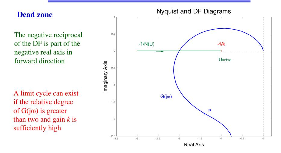
The oscillation frequency is the critical frequency  $\omega_c$  of the linear system and the oscillation magnitude depends on the dead zone parameters  $\beta$  and *k*
