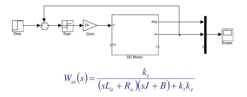
The linear plant is characterised by an all-pole transfer function with relative degree two, therefore there is no contact point between the Nyquist plot and the real negative axis, but the origin at  $\omega = +\infty$  (corresponding to U=0 in the DF plot)
