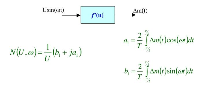
The evaluation of coefficients  $a_1$  and  $b_1$  can be performed by means of both analytical calculation and numerical integration, depending on the type of nonlinearity involved
