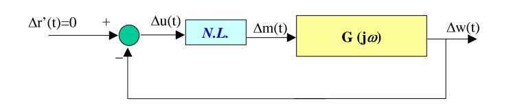
If the block N.L is a pure constant k, the stability of the feedback system can be performed by means of the Nyquist criterion, which gives the number of roots with positive real roots of the Harmonic Balance Equation
