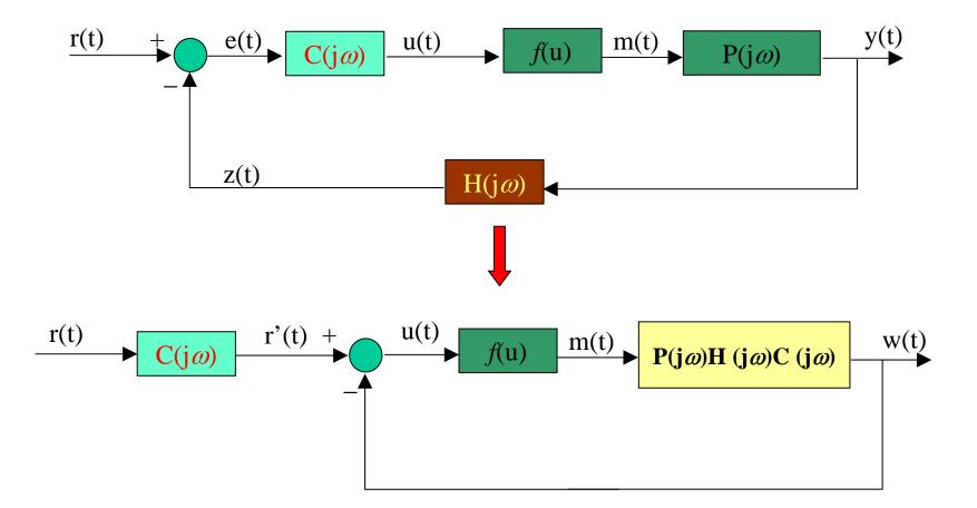
If constant (or very slowly varying) reference signals are considered, under some conditions it is possible to separate the low-frequency, almost static, behaviour defined by a working nominal condition and a highfrequency behaviour due to small variations around such a working point
