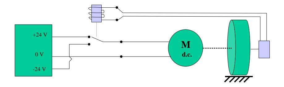
The position of the motor shaft is measured by means of a rotational variable resistance.
