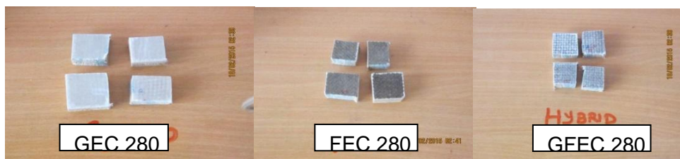
Fig 5.3 Sandwich structures with cork density 280\text{kg/m}^3
