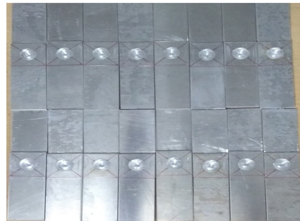
Fig. 4 – Photograph of AA6061-T6/Al 2 O 3 SFSSW welded samples.
