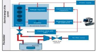
Fig. 1: E-Nose System Design
