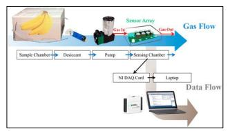
Fig. 7: E-Nose System for Analysing Aroma in Fruits
