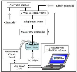
Fig. 8: E-Nose System for Fishing Industry
