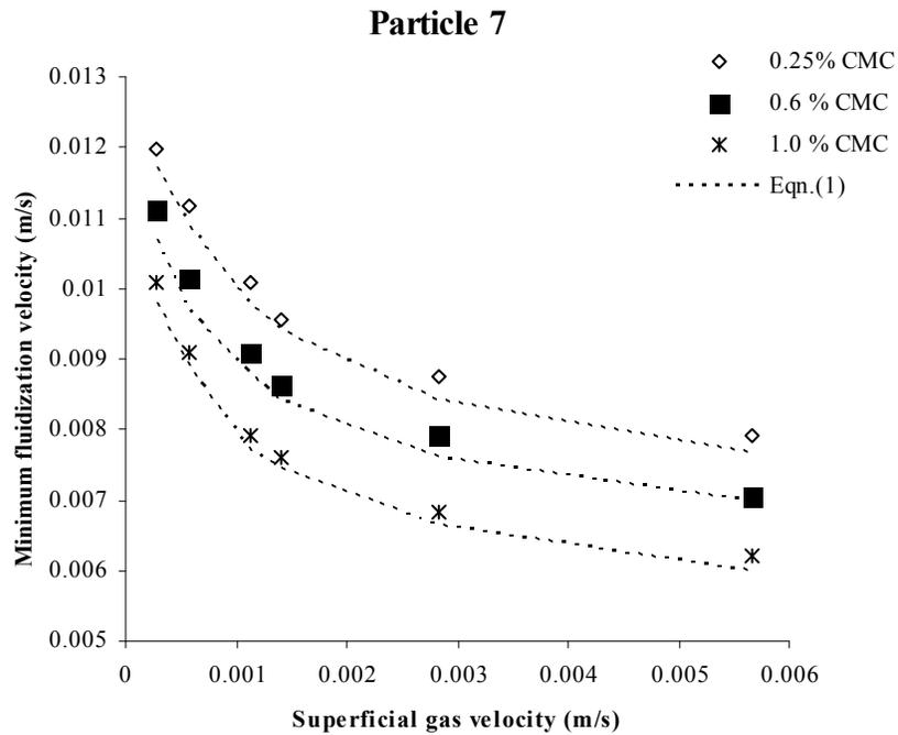
Fig.7 Effect of rheological properties on Minimum fluidization velocity
