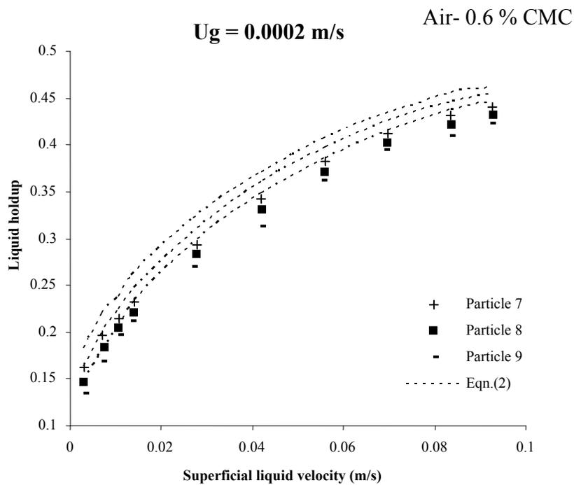
Fig.10 Effect of particle sphericity on liquid holdup
