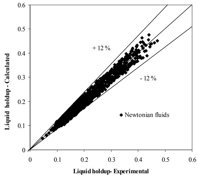
Fig.20 Comparison between the Experimental and Calculated Values of Liquid holdup for Newtonian Liquids
