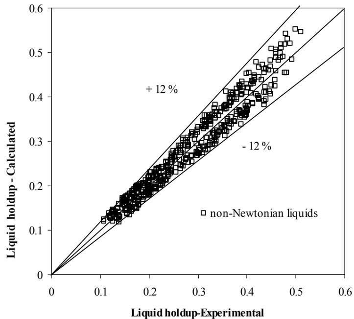
Fig.21 Comparison between the Experimental and Calculated Values of Liquid holdup for non-Newtonian Liquids
