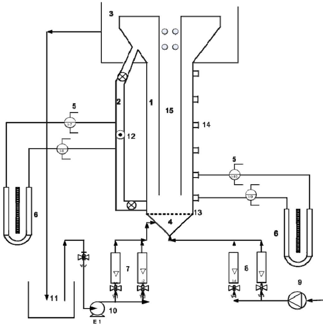
1. Riser, 2. Down comer, 3. Gas liquid Separator, 4. Calming section, 5. Gas liquid Separator for Manometer, 6. Manometer, 7. Rotameter for Liquid flow rate, 8. Rotameter for Gas flow rate, 9. Gas inlet valve, 10. Liquid circulating pump, 11. Liquid Storage tank, 12. Orifice, 13. Supporting Screen, 14. Manometer Tapings, 15. Draft tube.
