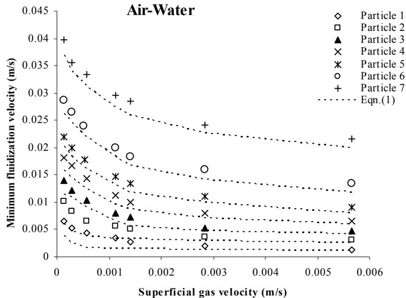
Fig.2 Effect of particle diameter on Minimum fluidization velocity
