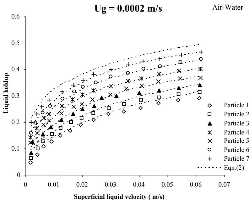
Fig.8 Effect of particle diameter on liquid holdup
