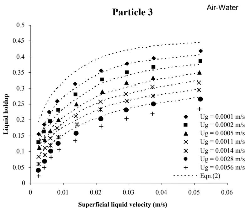
Fig.11 Effect of superficial gas velocity on liquid holdup
