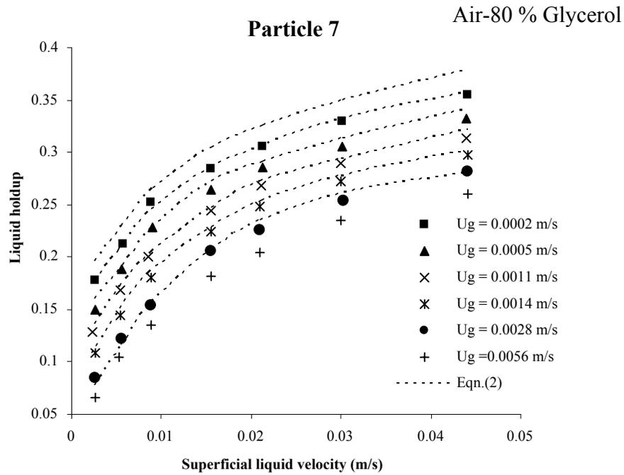
Fig.14 Effect of superficial gas velocity on liquid holdup
