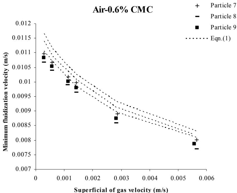
Fig.5 Effect of particle sphericity on Minimum fluidization velocity
