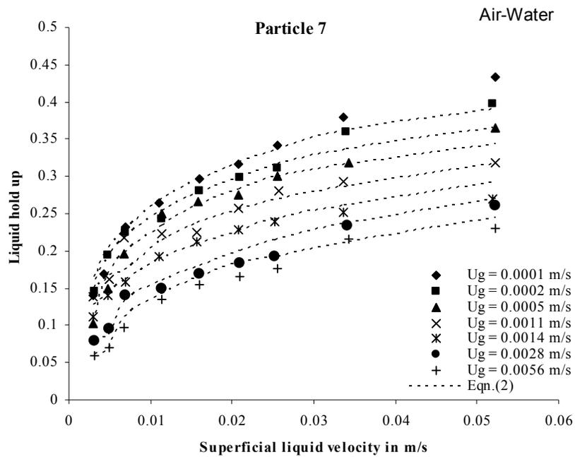
Fig.12 Effect of superficial gas velocity on liquid holdup
