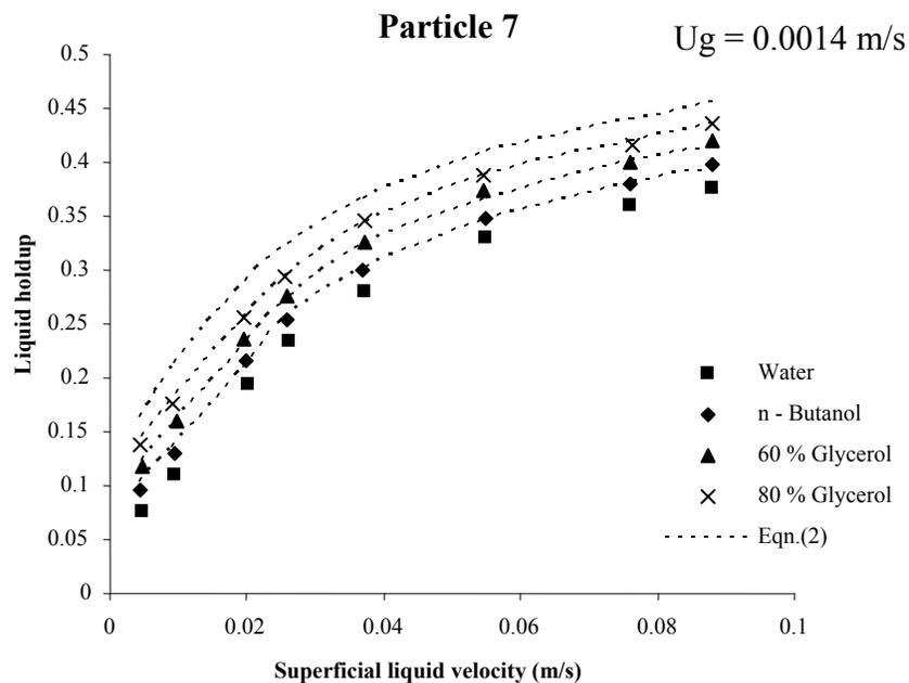
Fig.16 Effect of physical properties on liquid holdup
