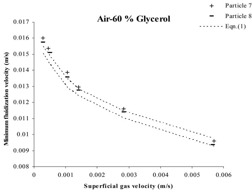
Fig.4 Effect of particle sphericity on Minimum fluidization velocity
