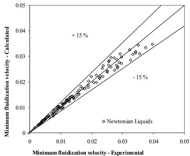
Fig.18 Comparison between the Experimental and Calculated Values of Minimum Fluidization Velocity for Newtonian Liquids
