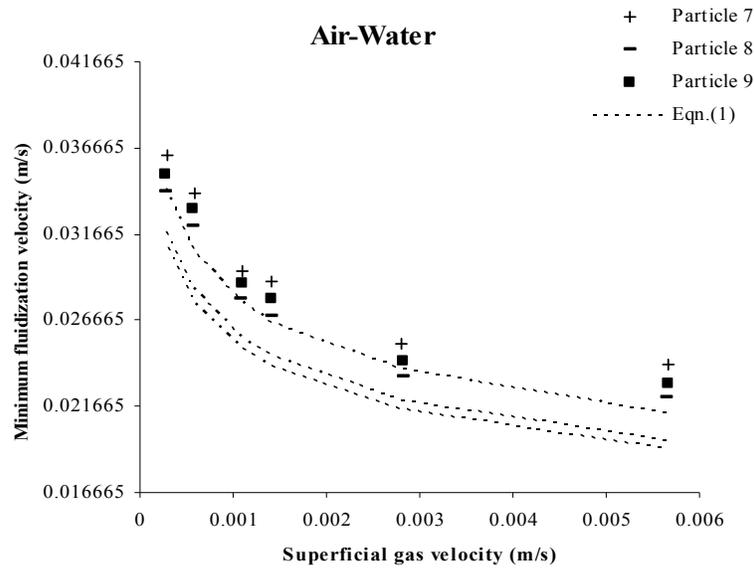
Fig.3 Effect of particle sphericity on Minimum fluidization velocity
