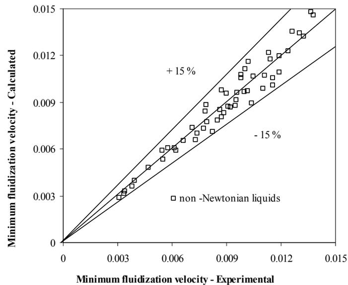
Fig.19 Comparison between the Experimental and Calculated Values of Minimum Fluidization Velocity for non-Newtonian Liquids
