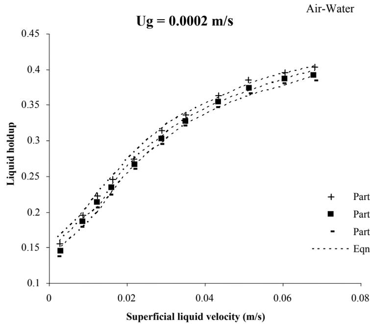
Fig.9 Effect of particle sphericity on liquid holdup
