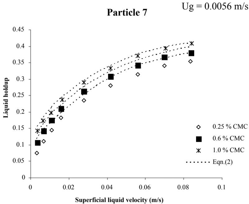
Fig.17 Effect of rheological properties on liquid holdup
