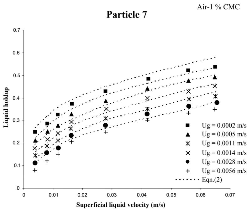
Fig.15 Effect of superficial gas velocity on liquid holdup
