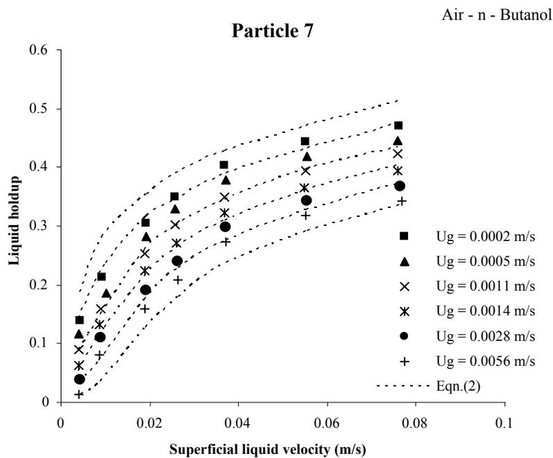
Fig.13 Effect of superficial gas velocity on liquid holdup
