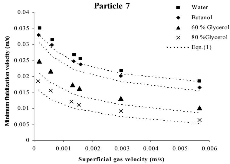
Fig.6 Effect of physical properties on Minimum fluidization velocity
