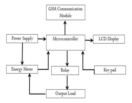
Fig. No: 1. Block diagram of Proposed system
