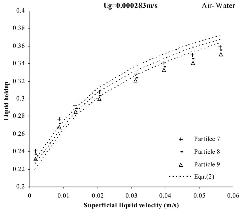
**Figure 12.**Effect of particle sphericity on liquid holdup
