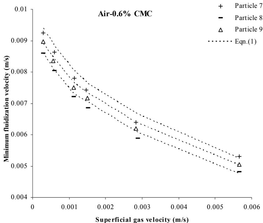
**Figure 4** .Effect of particle sphericity on minimum fluidization velocity
