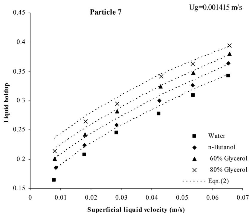
**Figure 14.**Effect of physical properties of Newtonian liquids on liquid holdup
