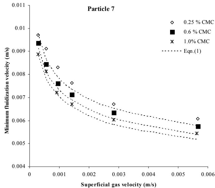
**Figure 6.**Effect of flow consistency index of non-Newtonian liquids on minimum fluidization velocity.
