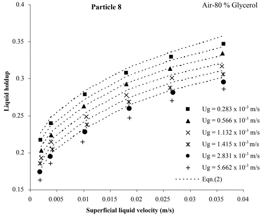
**Figure 9.**Effect of phase flow rates on liquid holdup for Air-80% Glycerol system
