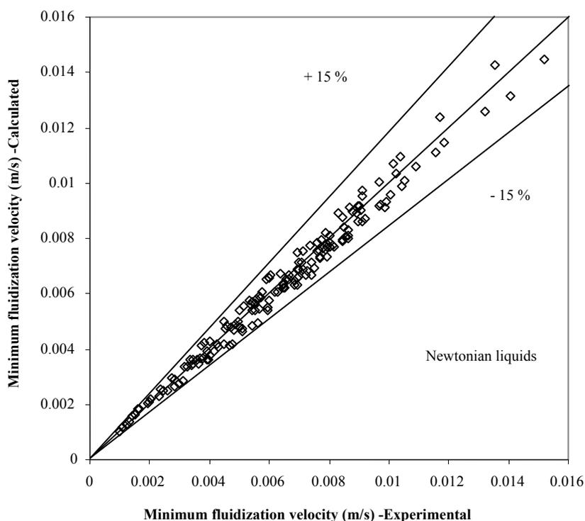
**Figure 17.** Comparison between the experimental and calculated values of minimum fluidization velocity for Newtonian liquids
