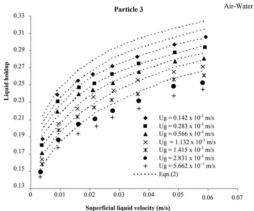
**Figure 7.**Effect of phase flow rates on liquid holdup
