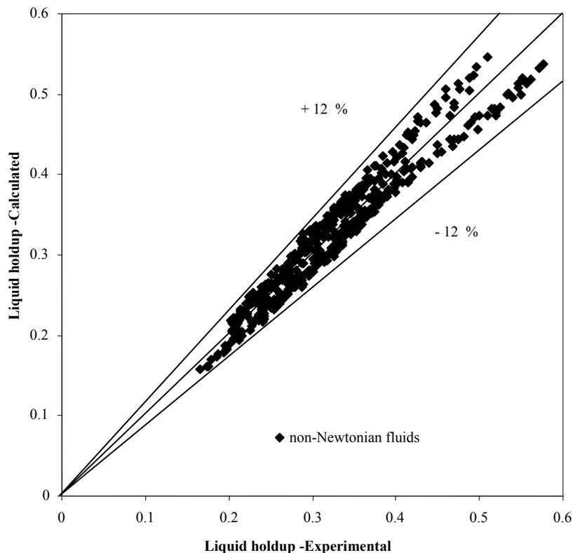
**Figure 20.** Comparison between the experimental and calculated values of liquid holdup for non-Newtonian liquids
