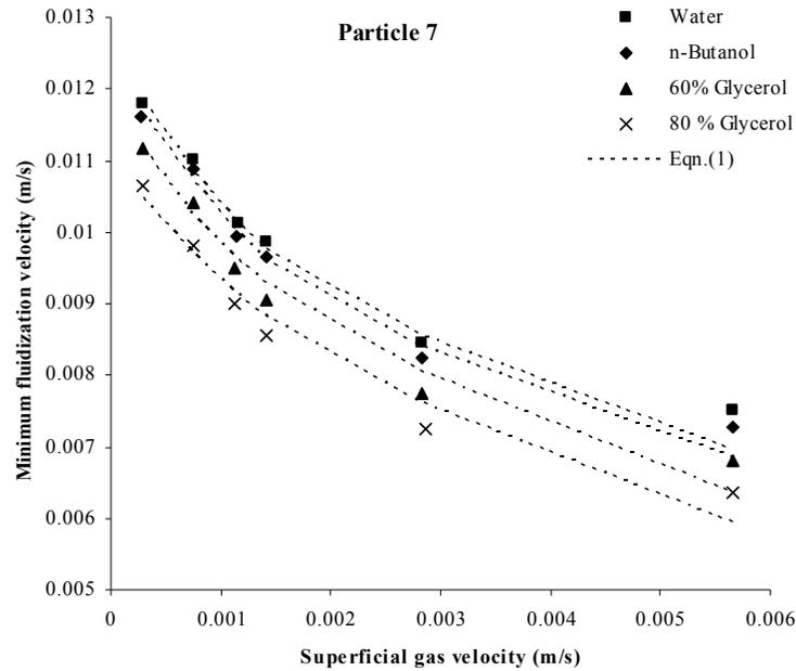
**Figure 5.**Effect of physical properties of Newtonian liquids on minimum fluidization velocity.
