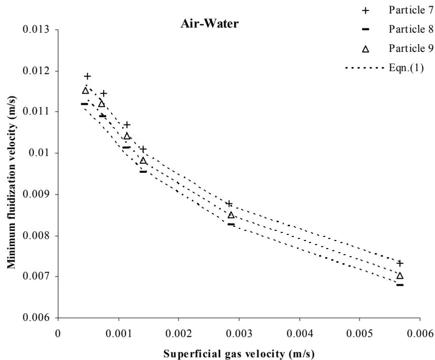
**Figure 3** .Effect of particle sphericity on minimum fluidization velocity
