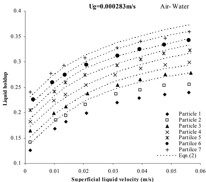
**Figure 11.**Effect of particle diameter on liquid holdup
