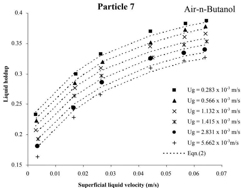
**Figure 8.**Effect of phase flow rates on liquid holdup for Air-n-Butanol system
