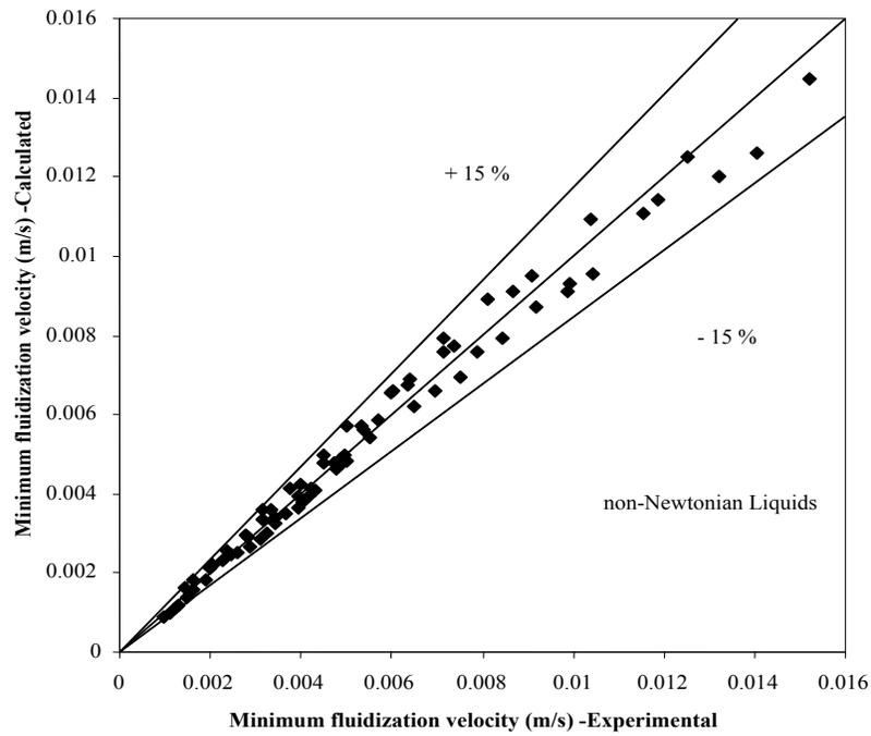
**Figure 18.** Comparison between the experimental and calculated values of minimum fluidization velocity for non-Newtonian liquids
