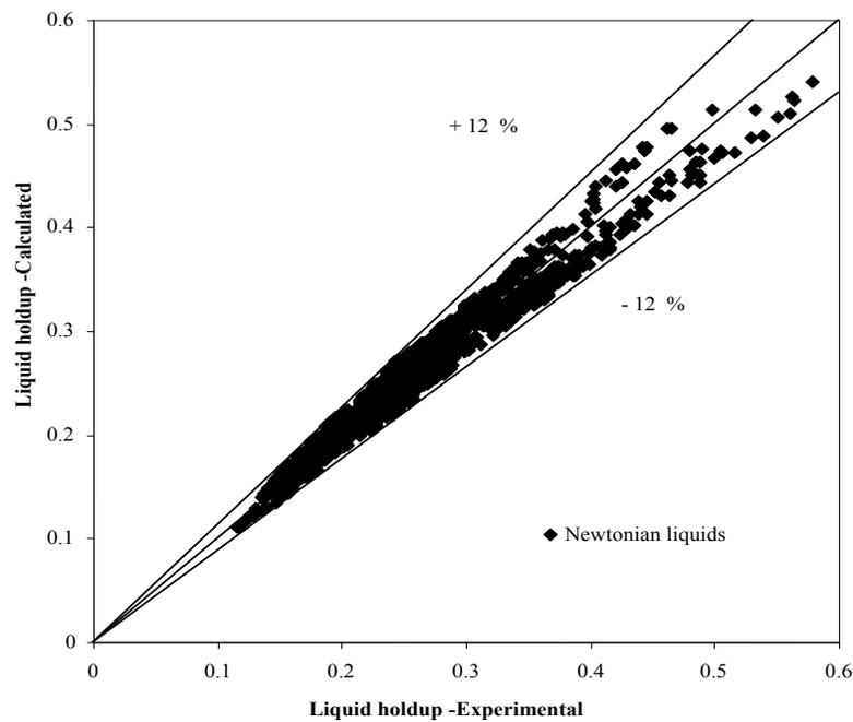
**Figure 19.** Comparison between the experimental and calculated values of liquid holdup for Newtonian liquids
