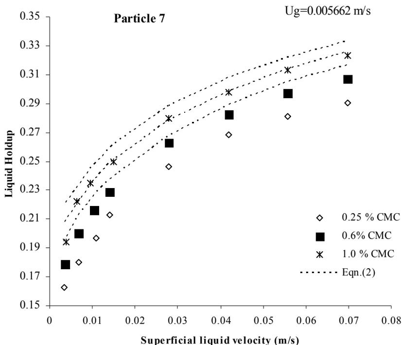
**Figure 16.**Effect of flow consistency index of non-Newtonian liquids on liquid holdup
