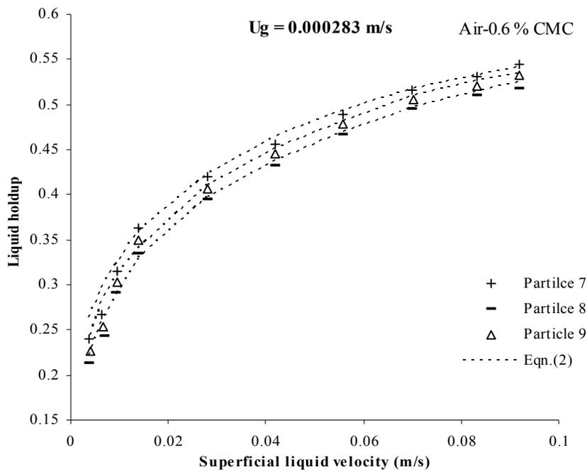
**Figure 13.** Effect of particle sphericity on liquid holdup
