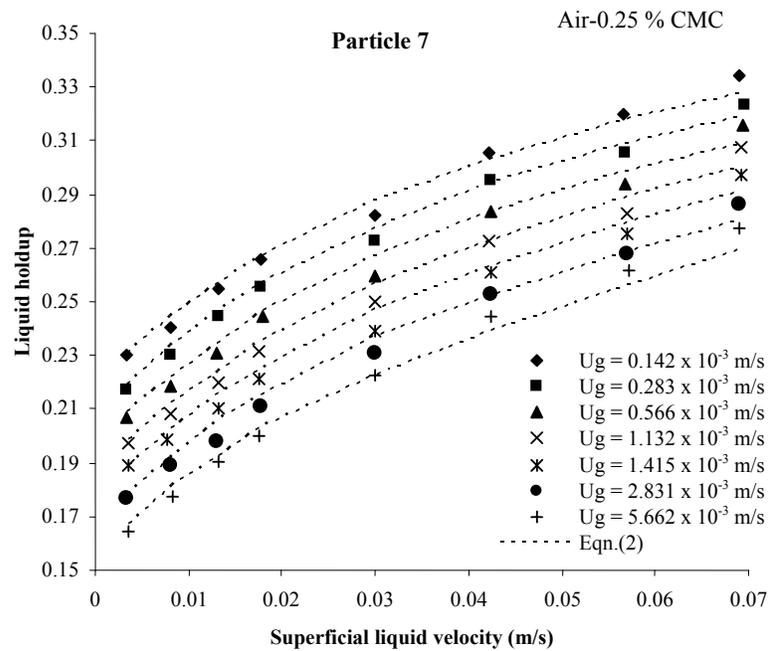
**Figure 10.**Effect of phase flow rates on liquid holdup for Air-0.25% CMC
