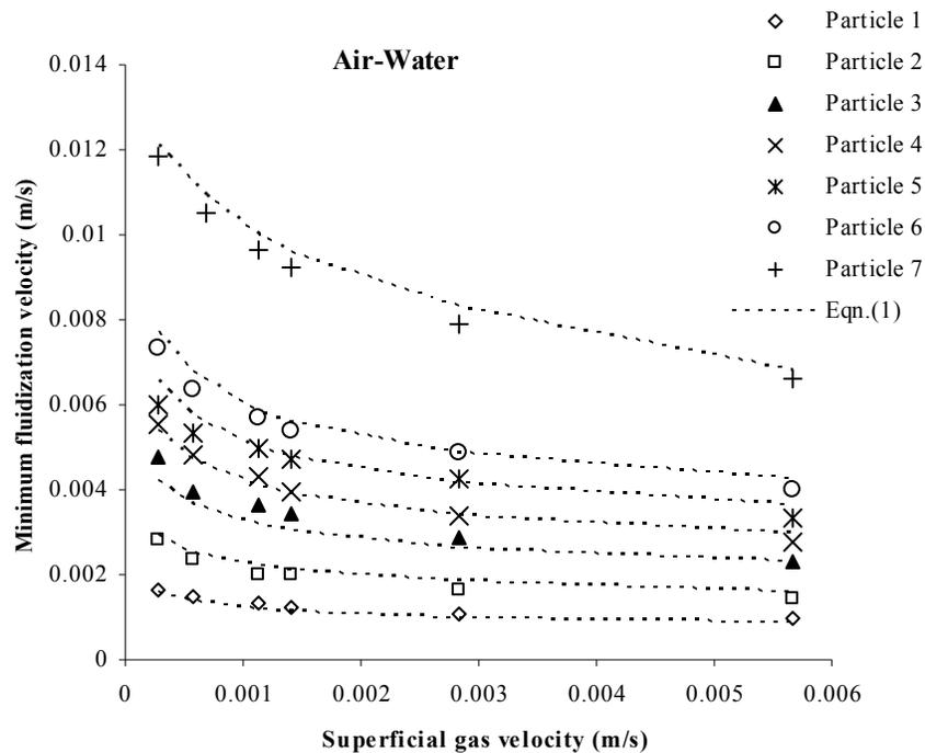
**Figure 2** .Effect of particle diameter on minimum fluidization velocity
