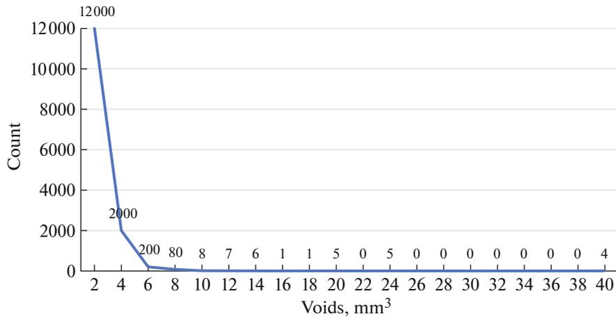
Fig. 3. Histogram of the void size distribution of the ETC concrete sample.
