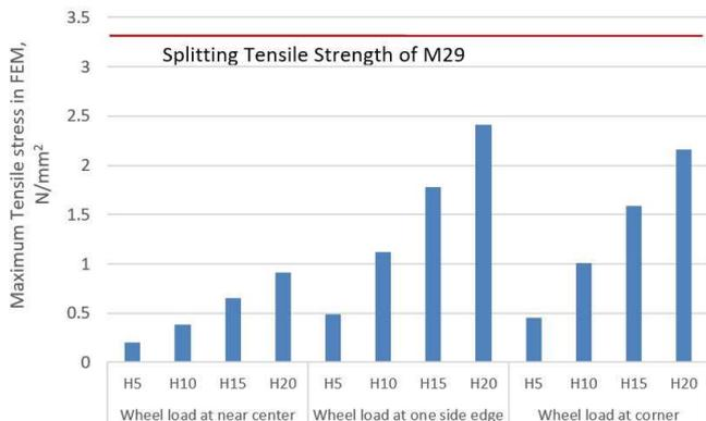
Fig. 15 – Comparison of Tensile Strength
