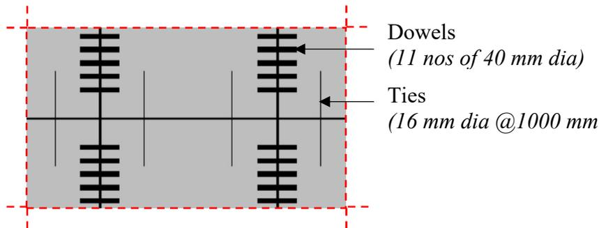
Fig. 8 - Specifications for slab joints
