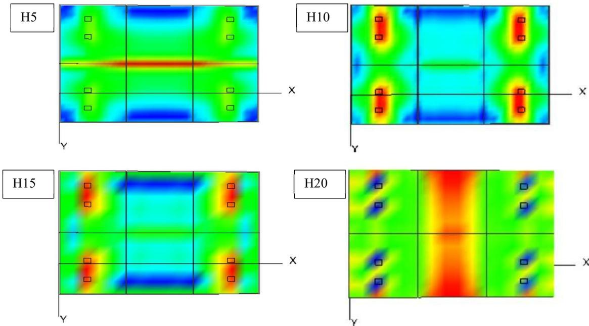
Fig.10- Stress distribution pattern on the pavement with near centre wheel
