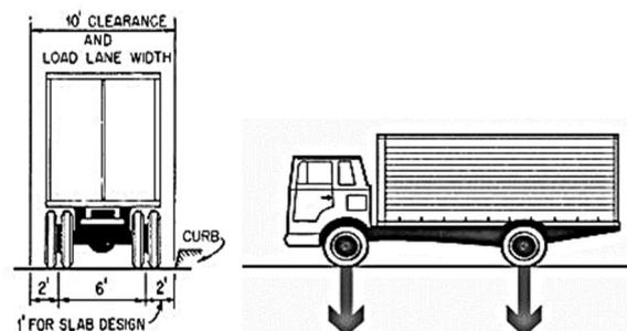
Fig.5 - Wheel load - Schematic representation
