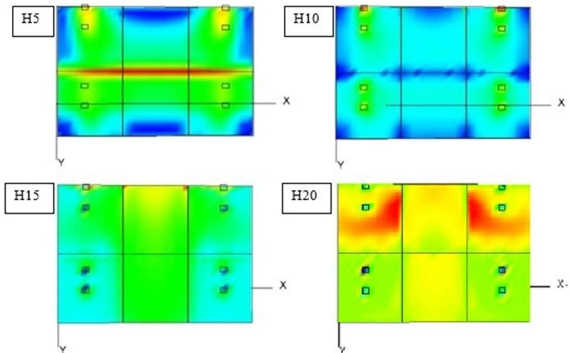
Fig. 11 - Stresses for wheel load at one side edge
