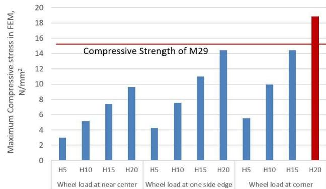
Fig. 14 – Comparison of Compressive Strength
