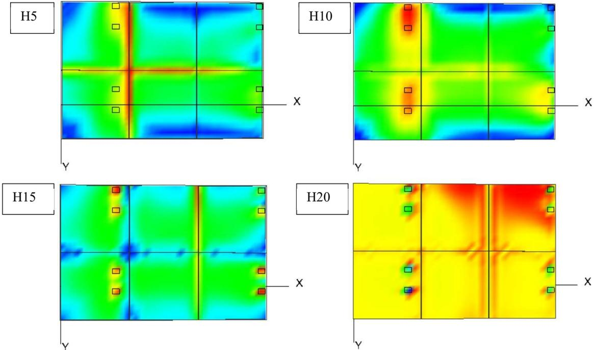
Fig. 12 – Stresses for wheel load at corner
