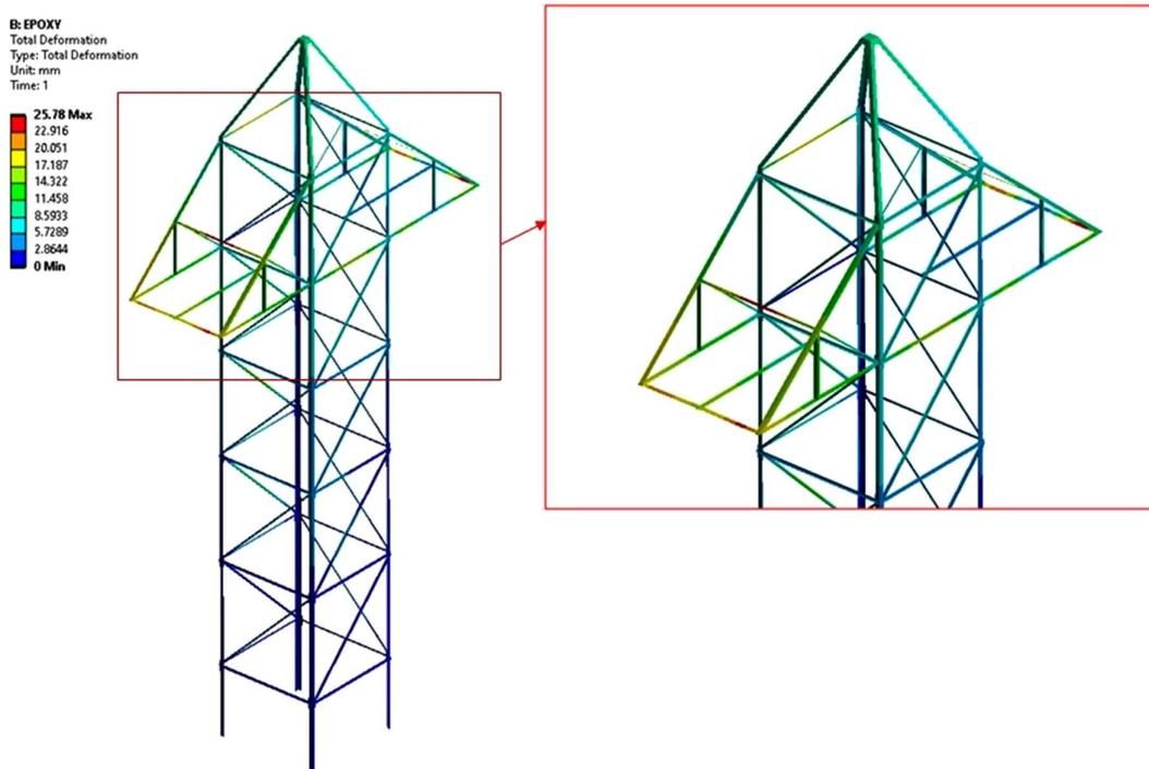
**FIG. 14** Deflection of GFRP transmission line tower with hybrid connection.
