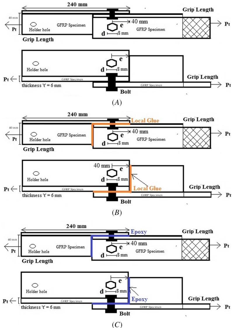
of hardener, and it will be fully mixed. The epoxy resin is applied between the connected two plates sections, and the bolt is tightened again.
