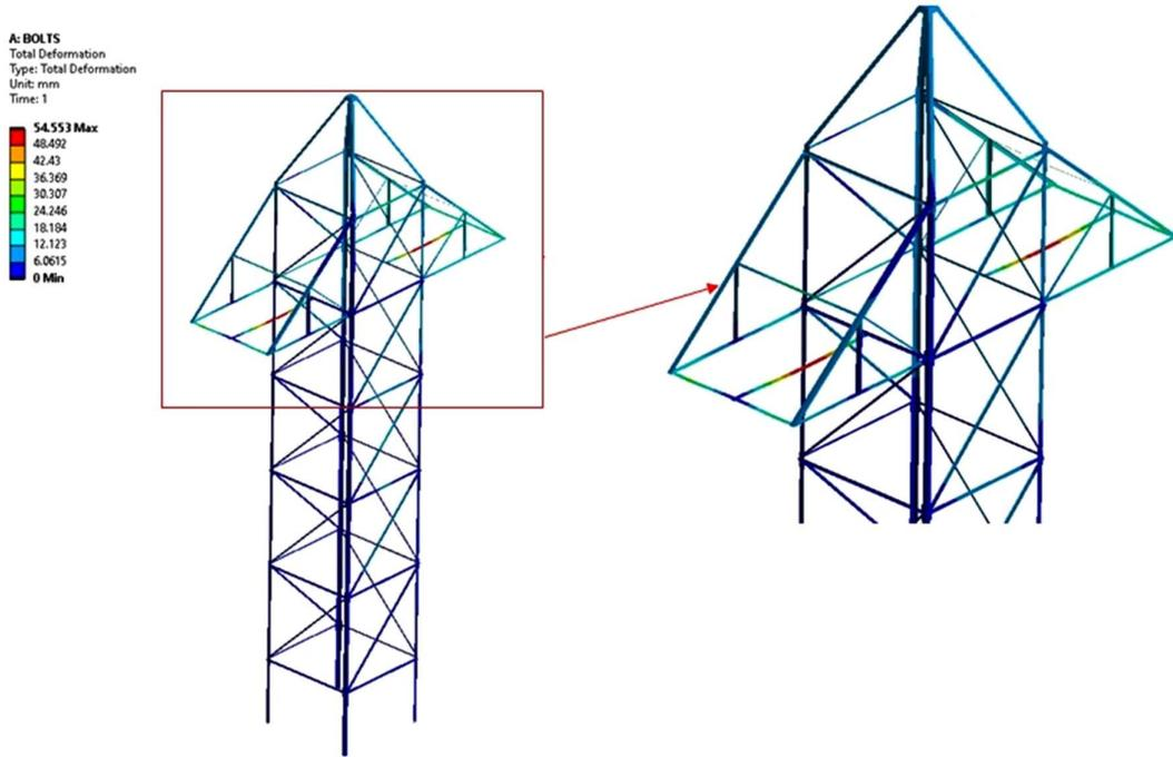
FIG. 13 Deflection of GFRP transmission line tower with adhesive connection.
