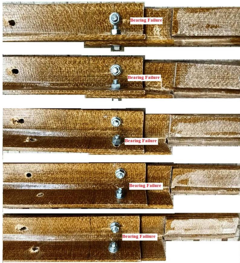
In the angle-to-angle bolted connections, 100 % of connected specimens only fail with bearing failure, whereas in the hybrid (local glue) and hybrid (epoxy) connections, 20 % of connected specimen fails were shear-out failure with maximum failure loads, and 80 % of connected specimen fails were bearing failure with maximum failure loads. The elongation percentage at peak load is also increased.
