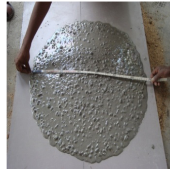
Fig. 1. Slump flow test
