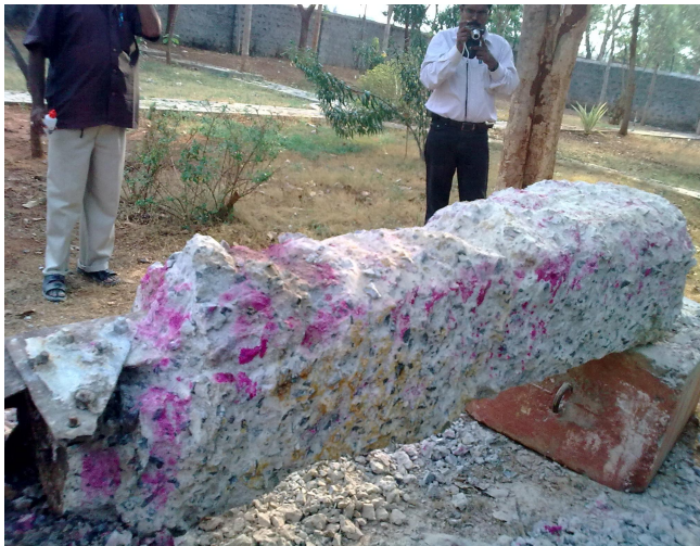
Fig.7 a. Spray of phenolphthalein on the specimen
