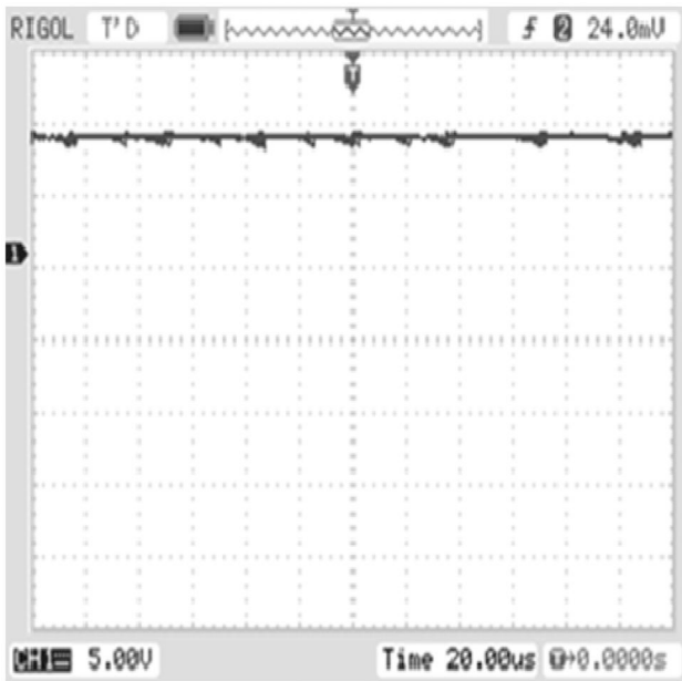
Figure 36. Voltage across battery during open-end X-Y read and head frame.
