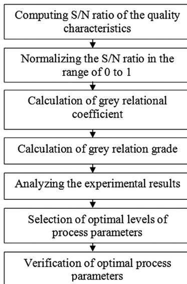
**Figure 1.** Flow chart showing the various steps followed in grey-based Taguchi method.
