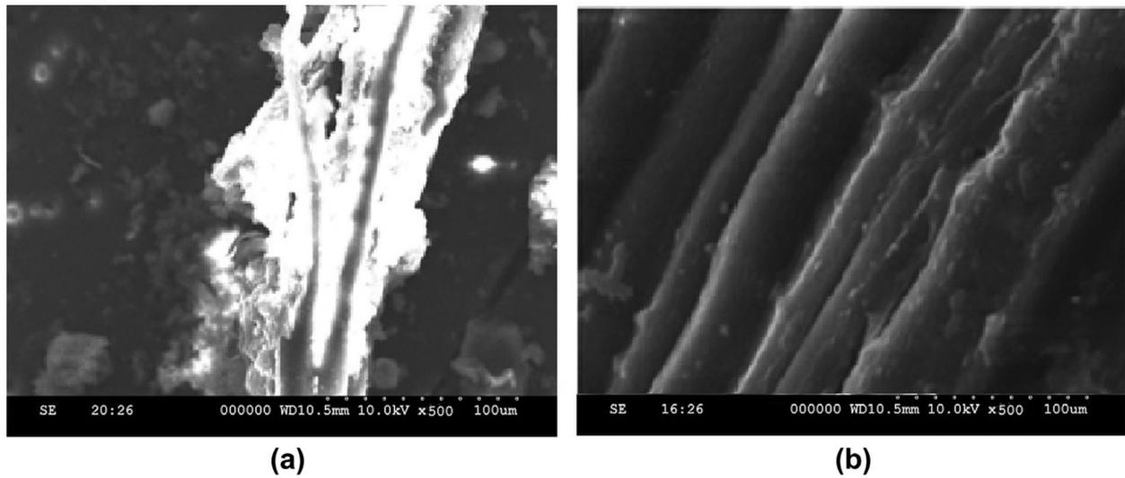
Figure 4. SEM image (x500) of fractured surfaces of composites (a) before tensile test (b) after tensile test.
