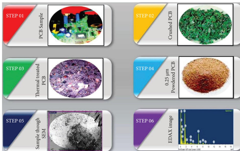
FIGURE 1: Schematic diagrams of primary raw PCBs into stepwise size reduction under the various mechanical operations and metal composition analysis performed by SEM with EDAX (reproduced from Murugesan et al., [31] under https://creativecommons.org/licenses/by/4.0 ).
