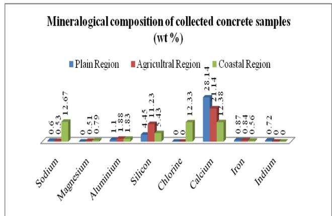
**Fig. 7. Mineralogical composition of tower footing concrete sample**
