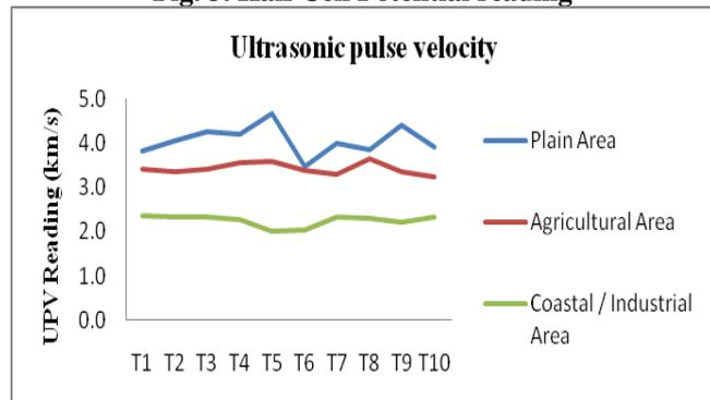
**Fig. 4. Ultrasonic pulse velocity**
