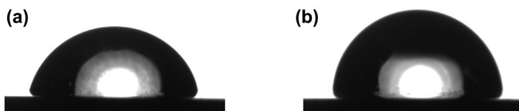
Figure 10. Contact angle images of (a) polished Cu and (b) API SAM modified Cu.
