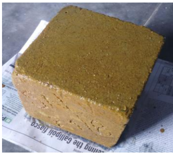
Fig. 9 Acid attack on cube
