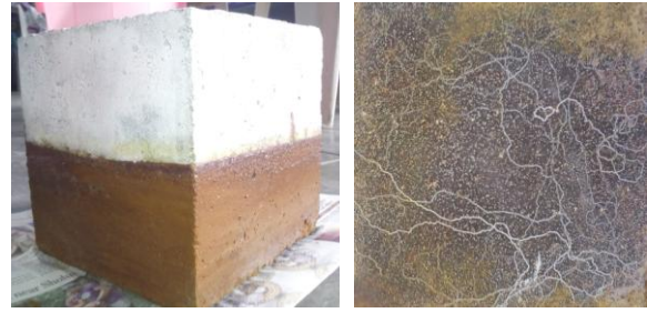
Fig. 10 Sulphate attack on cube
