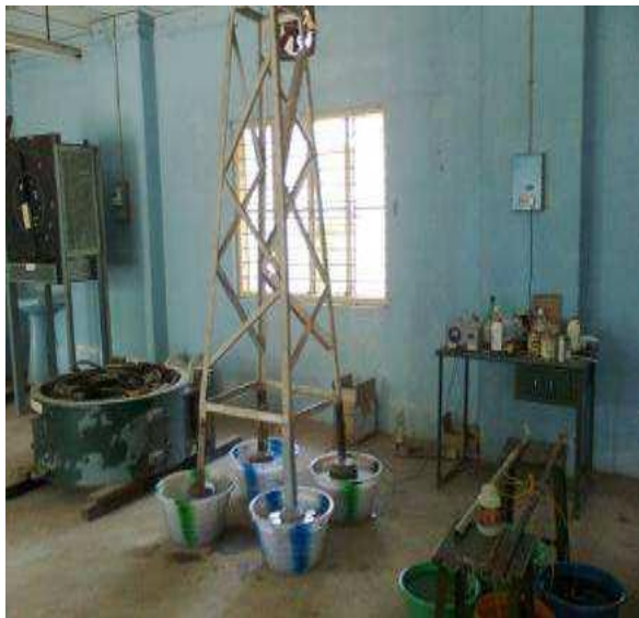
Figure 1. Model Tower foundation [Under corrosion acceleration]
