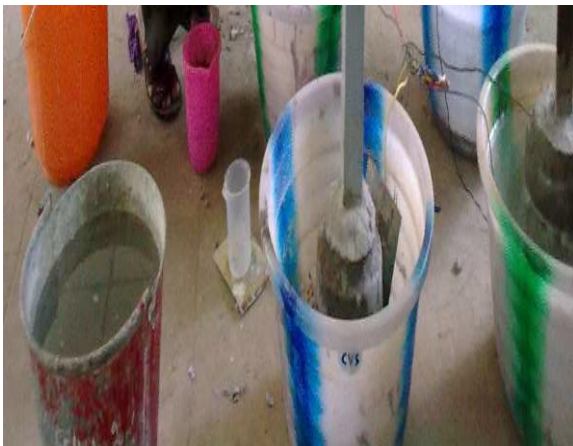
Figure 2. Close up view of leg of model tower [Casting of concrete around the stub angle and working in the crevice]
