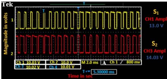
Fig. 14. Gate pulse and modulation signals using Xilinx Spartan 2-AN kit.
