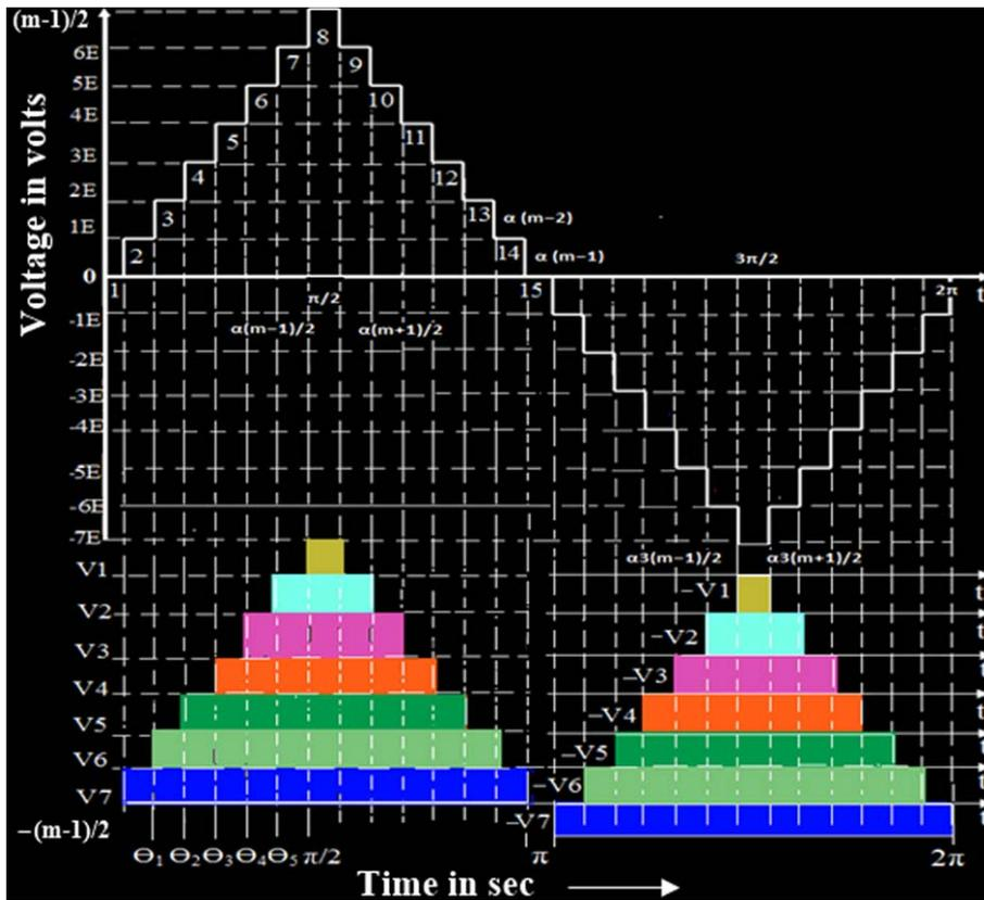
Fig. 6. Voltage Lift- Multilevel waveform of switching angle determination.
