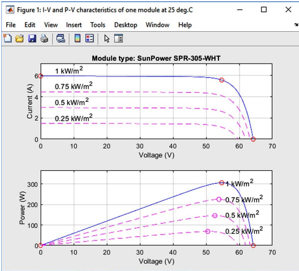
Fig. 3. Solar-PV Characteristics.
