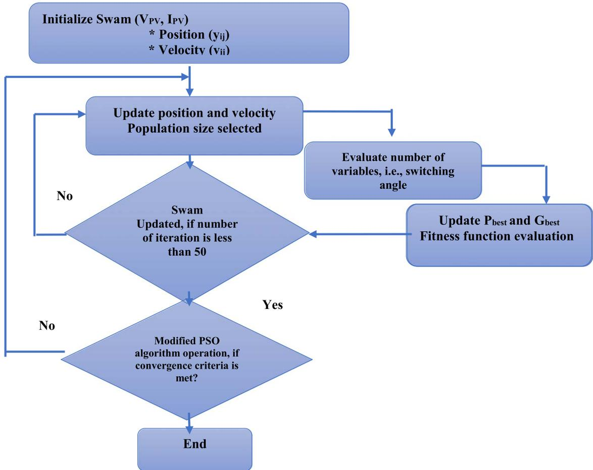
Fig. 7. Flowchart for MPSO implementation.
