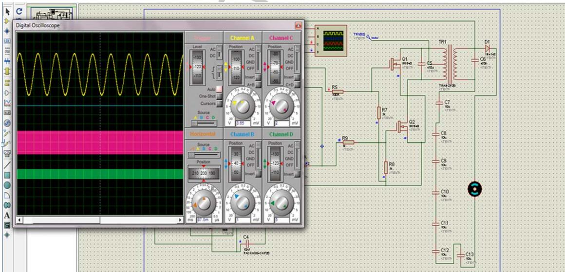
Fig. 9. Output voltage of 15-level VL-MLI.
