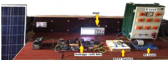
Fig. 13. Hardware setup for FPGA 3-AN Kit tuned Modified PSO algorithm.
