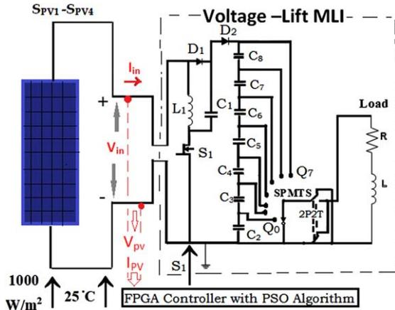
Fig. 1. Proposed Voltage-lift multilevel inverter.
