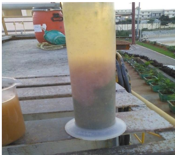
4.2: Sample after MBBR process at normal temperature condition.
