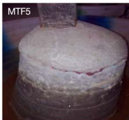
Fig.17. Deep pour grout o-rings after 500 hrs. of accelerated corrosion
