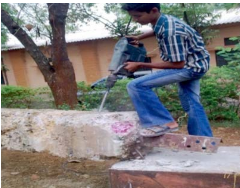
Fig.8. Close up view of coastal specimen on removal of stub concrete
