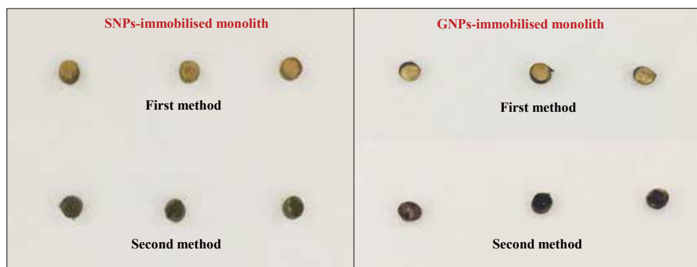
Fig. 4. Organic monolithic rod that was divided into three cross-sections (top, middle, and bottom) after immobilisation with NPs
