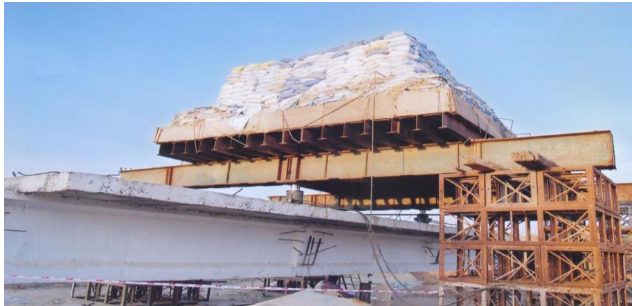
Fig. 3 Load test set up
