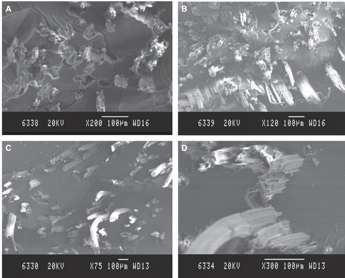
**Figure 4:** Scanning electron microscopy (SEM) image of fractured surface of tensile tested composite specimens: (A) experiment number=19, (B) experiment number=13, (C) experiment number=5 and (D) experiment number=16.
