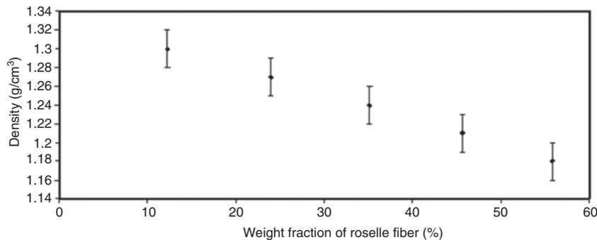
**Figure 2:** Variation of density with different weight percent of roselle fiber reinforced in vinyl ester resin matrix. [Fixed value: 0.02, percentage: 5, standard deviation (s): 1].
