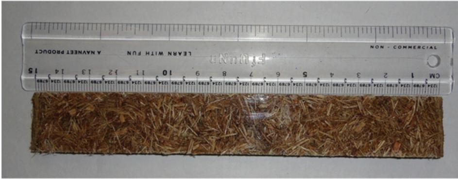
Figure 1: Digital image of composite specimens by hand lay-up method.
