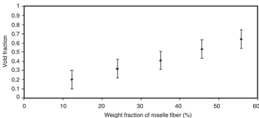
**Figure 3:** Variation of void fraction of composite with wt% of roselle fiber-reinforced vinyl ester composites. [Fixed value: 0.1, percentage: 5, standard deviation (s): 1].
