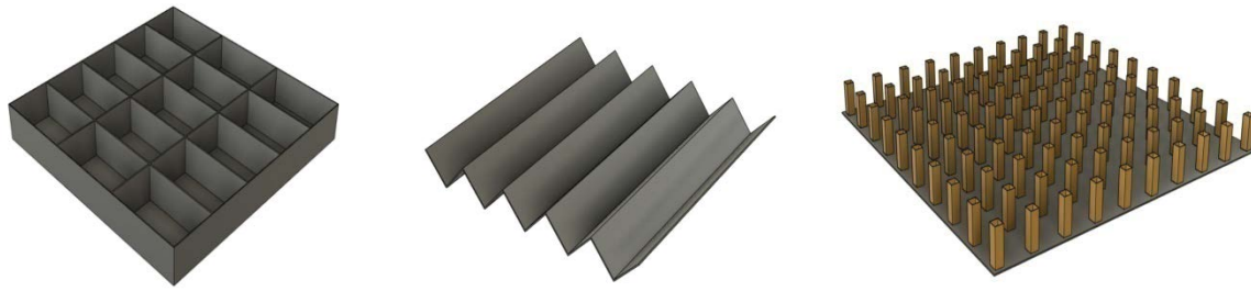
Fig. 4. Compartmental basin, corrugated basin and plain basin with fin.
