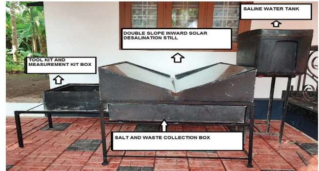
Fig. 3. V-type solar desalination still with experiment components.
