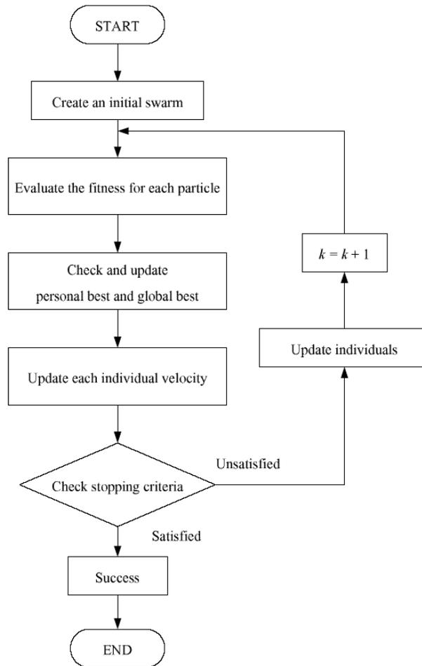
Fig. 4: Flowchart of PSO Algorithm
