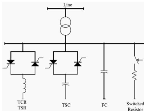
Fig. 1: Single Line Diagram of SVC
