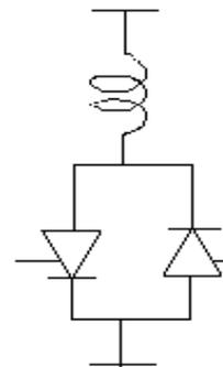
Fig. 2: Thyristor Controlled Reactor (TCR)
