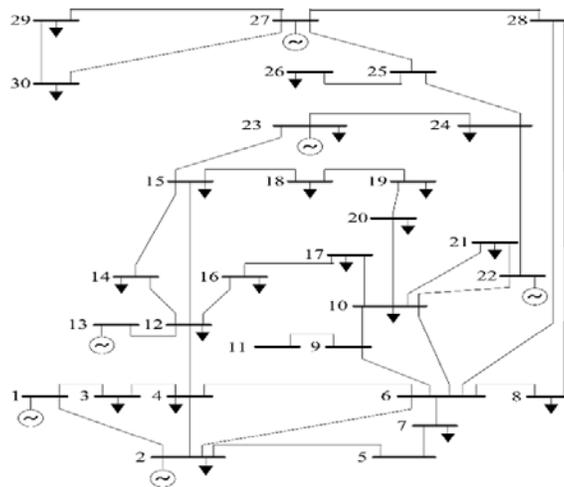
Fig. 5: Single Line Diagram of IEEE-30 Bus System
