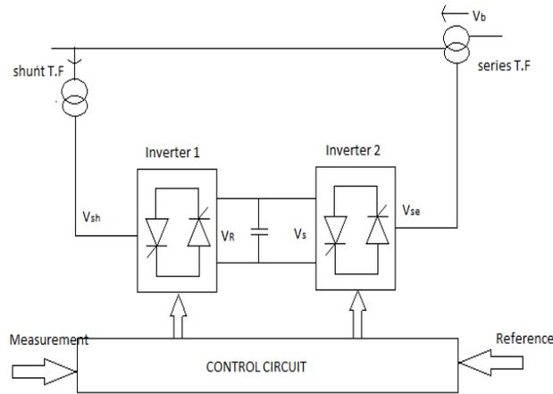
Fig. 3: Single Line Diagram of UPFC
