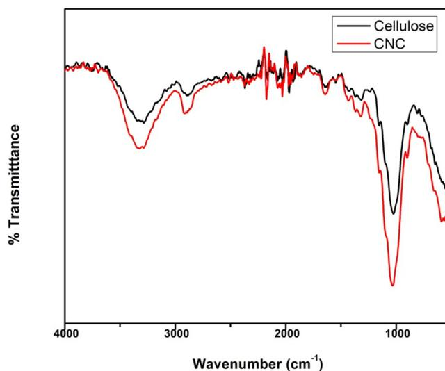
Fig. 4. ATR-FTIR spectra of (1)  $\alpha$ -cellulose (2) cellulose nanocrystal.
