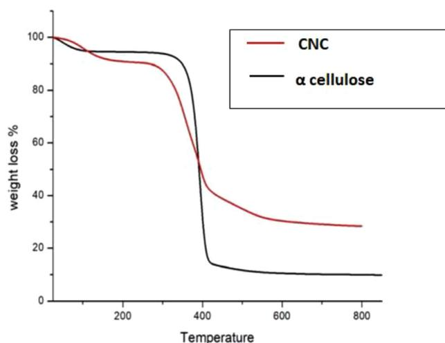
Fig. 7. TGA of alpha cellulose and cellulose nanocrystals.
