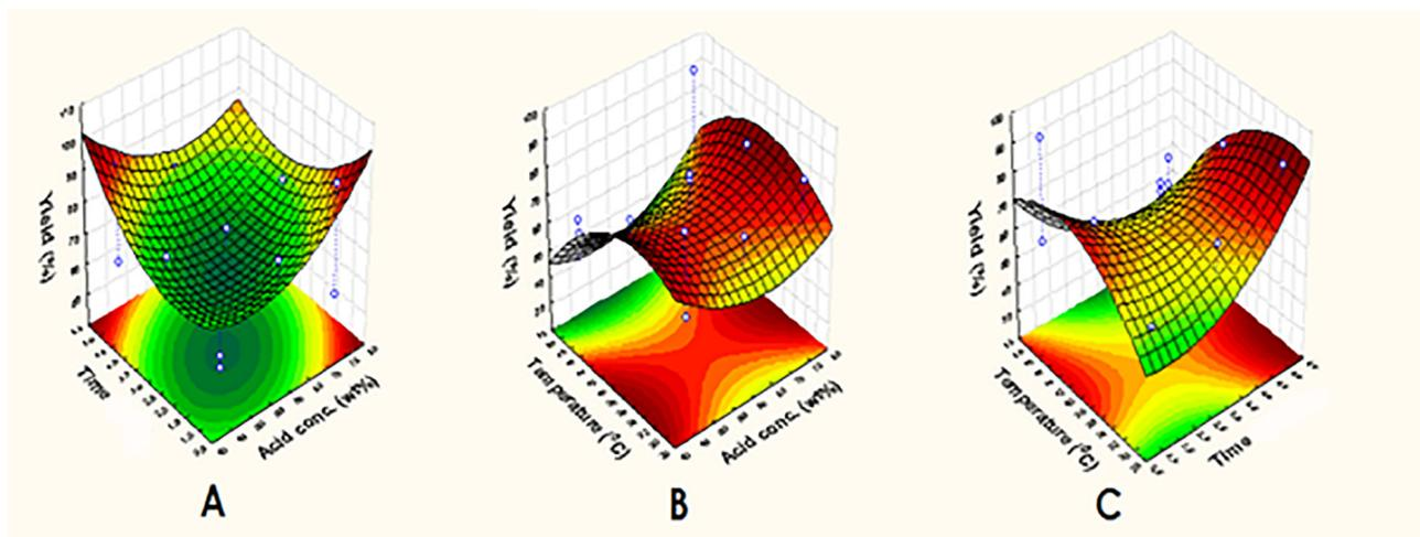
Fig. 2. (A) Contour plot between conc. of  $\text{H}_2\text{SO}_4$  (%) and Time (h); (B) Contour plot between conc. of  $\text{H}_2\text{SO}_4$  (%) and Temperature ( $^\circ\text{C}$ ); (C) Contour plot between Temperature ( $^\circ\text{C}$ ) and Time (h).
