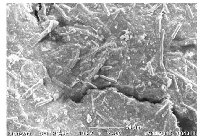
Fig. 3. SEM image of cellulose (rod like crystals).
