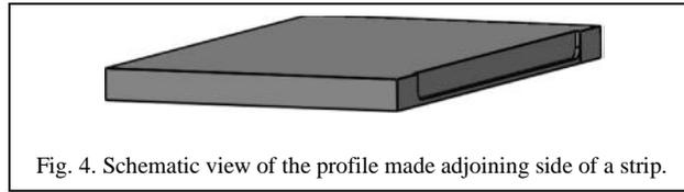
Fig. 4. Schematic view of the profile made adjoining side of a strip.
