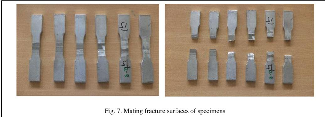
Fig. 7. Mating fracture surfaces of specimens
