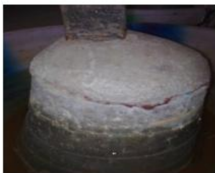
b. O-ring and Nano Zycosil coated surface
