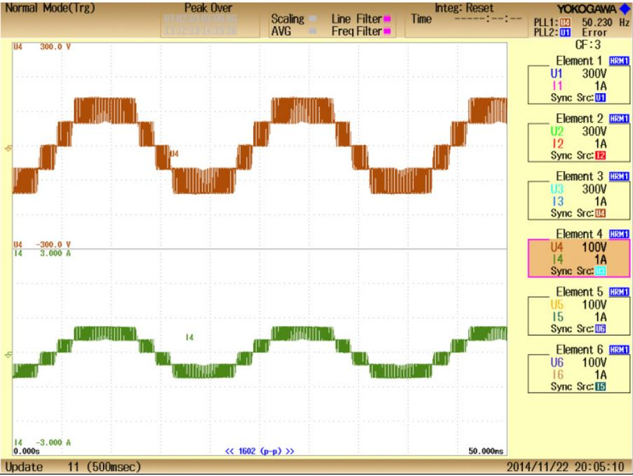
Fig. 15. Experimental result of MLI 5-level output voltage. Time base 5 ns/div.
