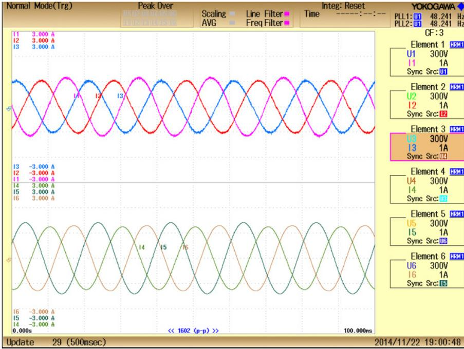
Fig. 13. Experimental result of grid current with 3-phase MLI Current. Time base 10 ns/div.
