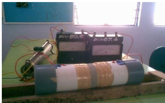
Fig. 2 — View of Rapid chloride penetration test set up
