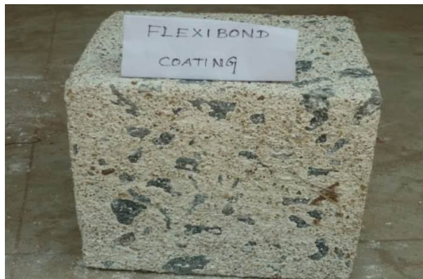
Fig. 5 — Deterioration of concrete due to acid attack
