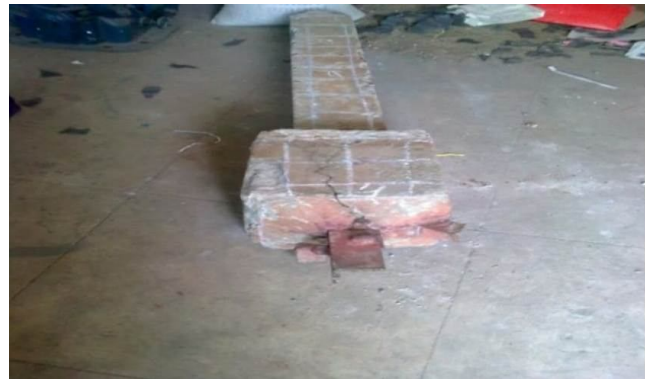
Fig. 13 — Stub excavated in Chennai (Marine environment)
