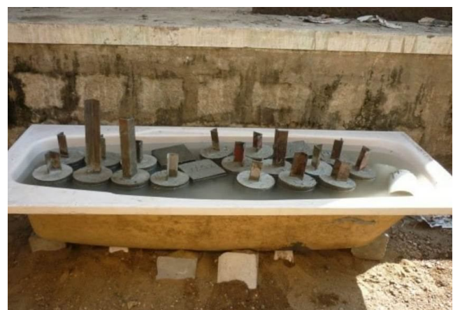
Fig. 1 — Curing of Testing Specimens
