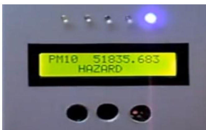
Fig 4: LCD display for pollution level
