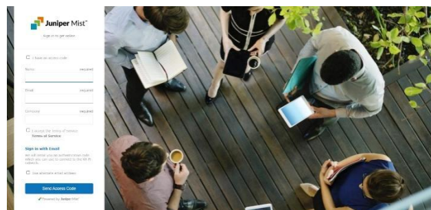
Fig. 2. Captive Portal Authentication Page for Guest Wireless Network Access using Juniper Mist Cloud.
